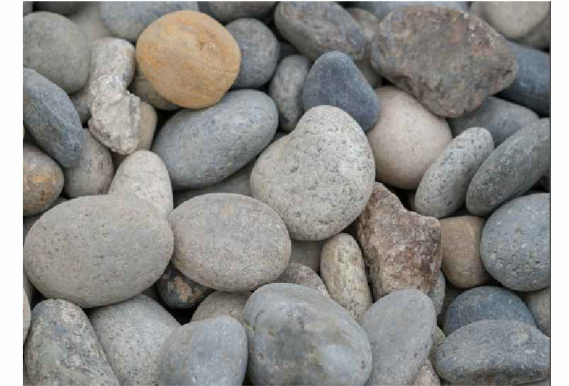
SANTA FE COBBLESTONE: Dry River Bed feature to be lined with stones ranging in size from 4" - 8" and filled with 1-3" stones.
