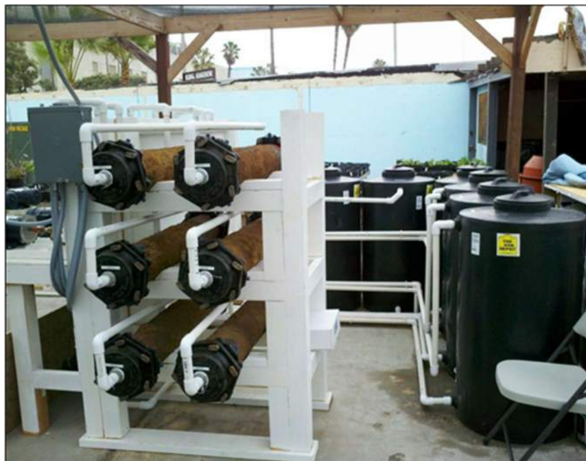
Figure 4-7: Example of Recirculation Pipe Loop System
