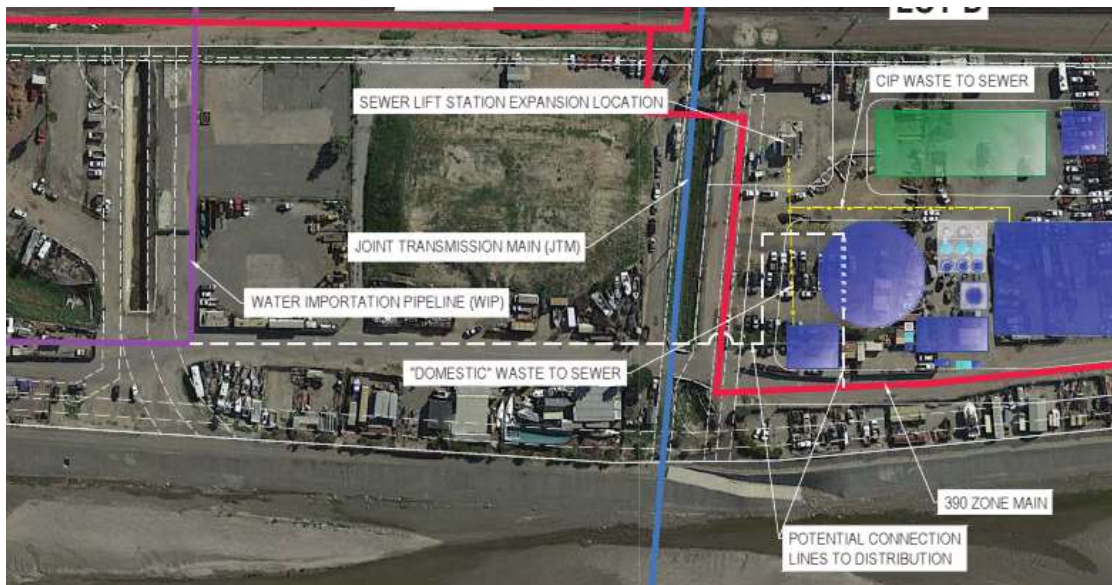
Figure 1-2: Regional Transmission Mains Near Proposed Doheny Site (PEIR, 2018)
