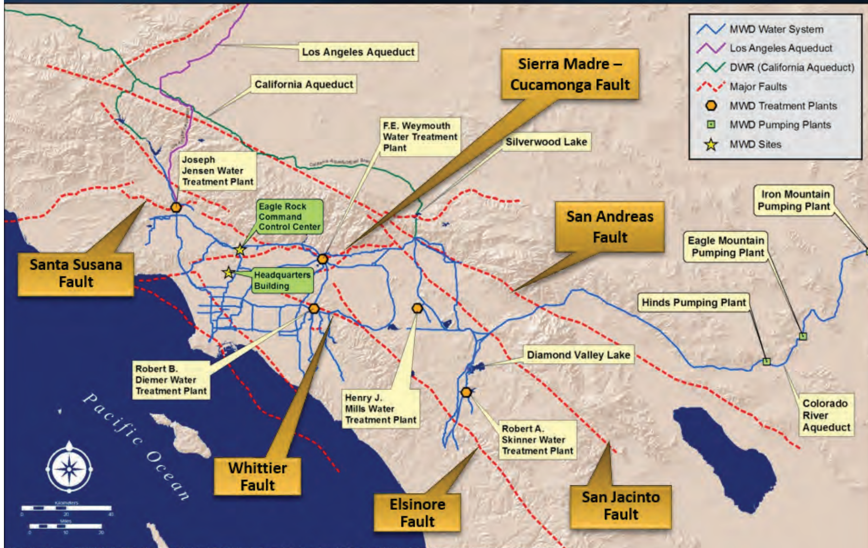
Figure 2 – Many Earthquake Faults pose risks to water delivery systems in Southern California
